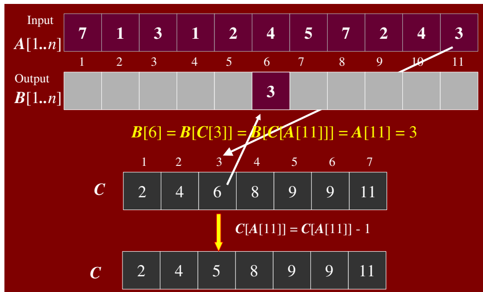
Figure 5.9: A[11] placed in output array B
