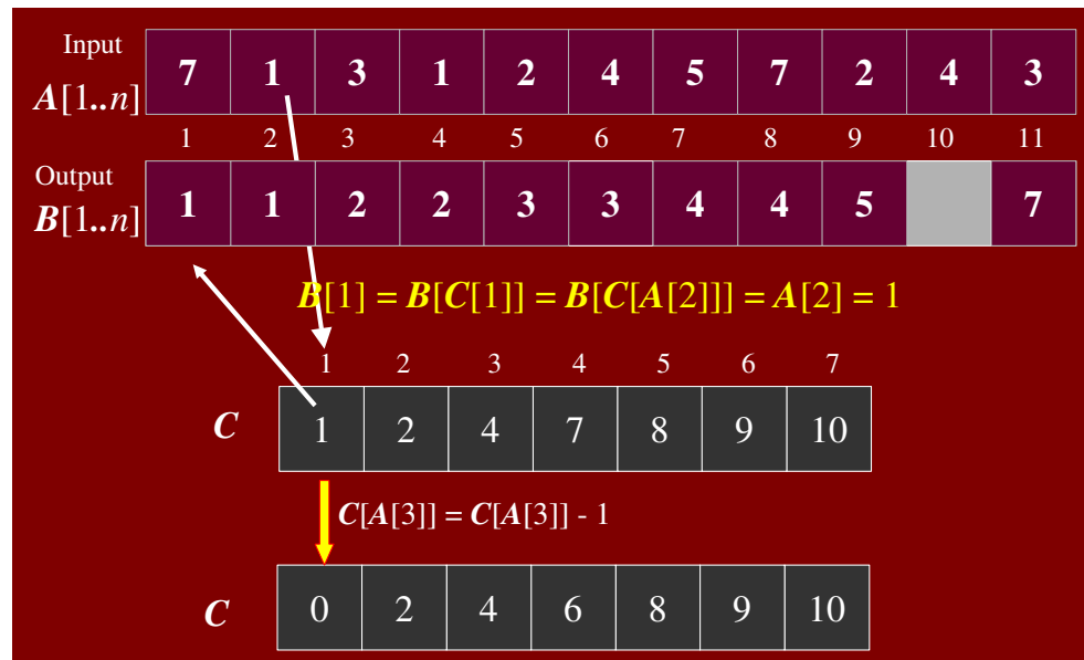
Figure 5.18: A[2] placed in output array B
